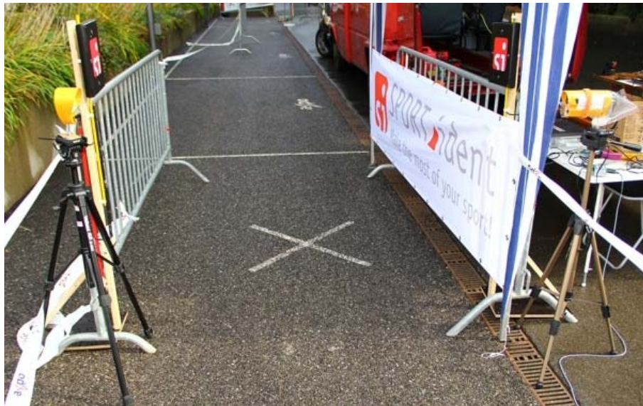
Picture 1: Gate mode configuration of the BS11 BL station at the finish line enables a very accurate measurement of finish times.
